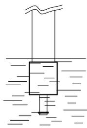
The contact is CLOSED when the float is in the liquid
