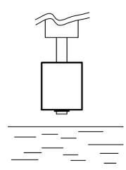
The contact is OPEN when float is above the liquid level.
